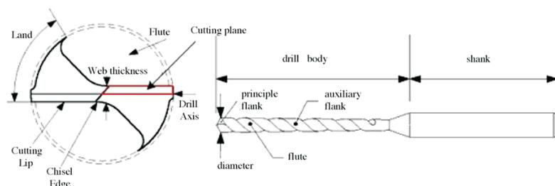
Fig.2. Schematic diagram of a microdrill [7]
