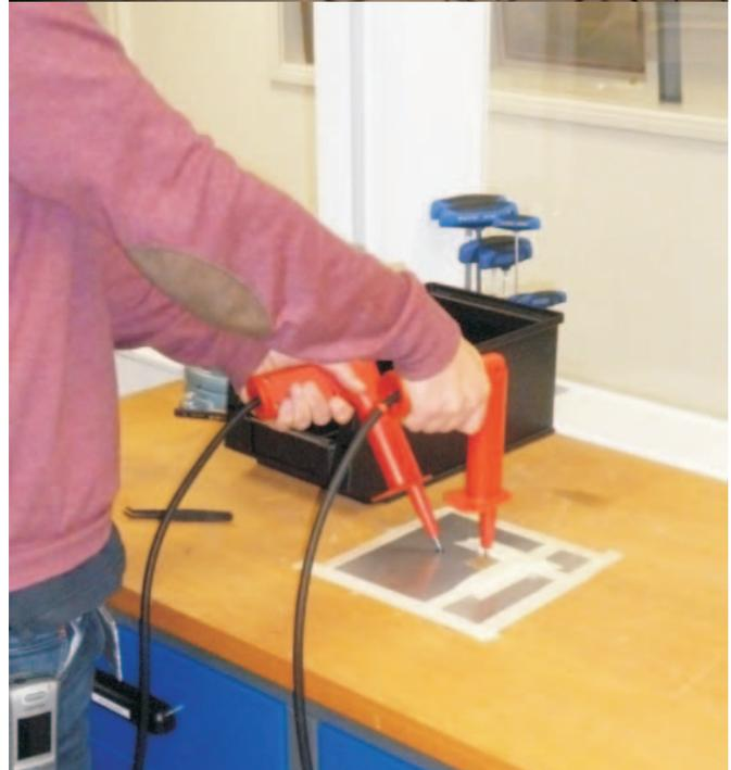
Figure 3: Dielectric breakdown test, high voltage is applied until arc occurs on the sidewall
